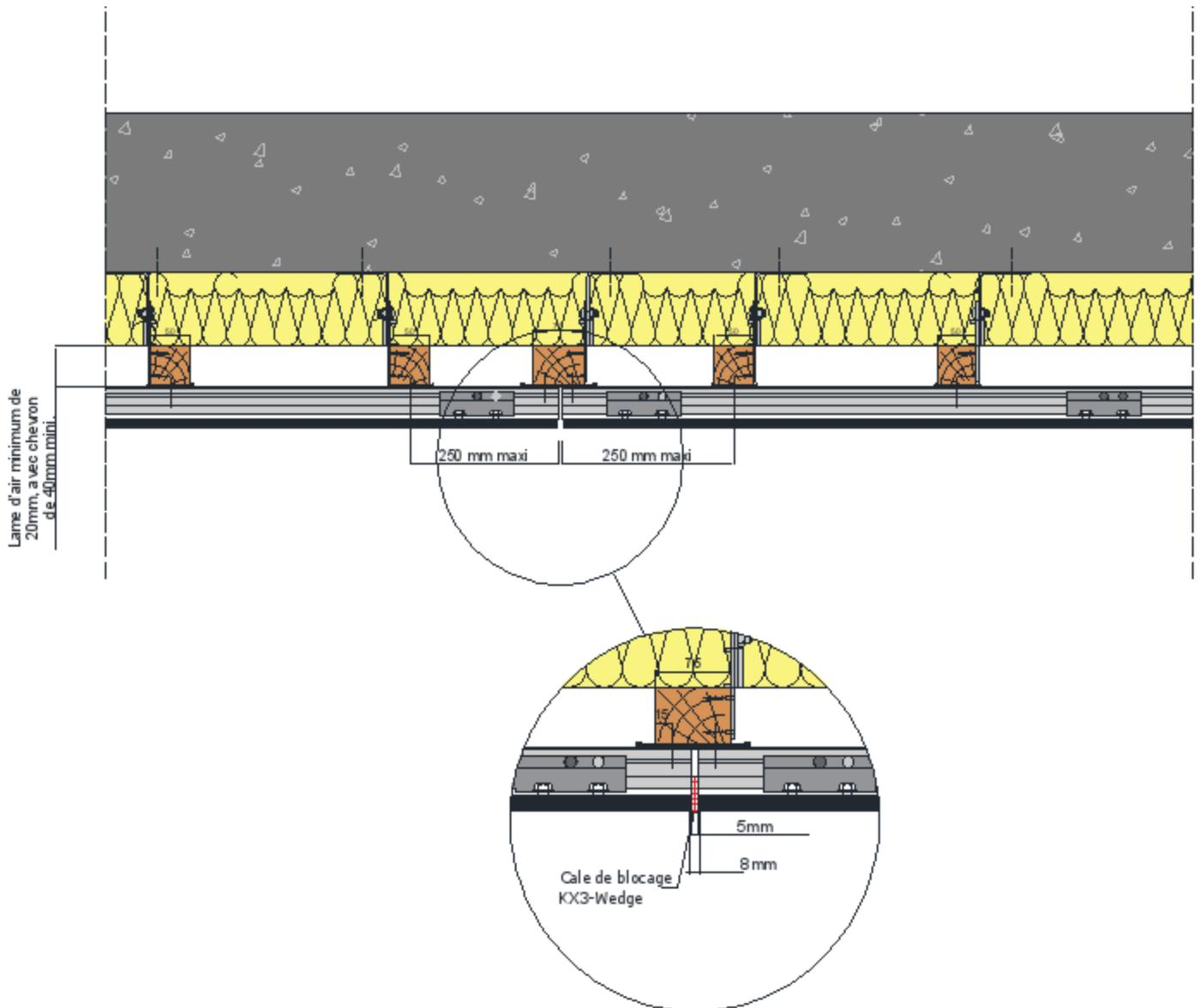
**Figure 15 - Joint vertical (coupe horizontale)**
