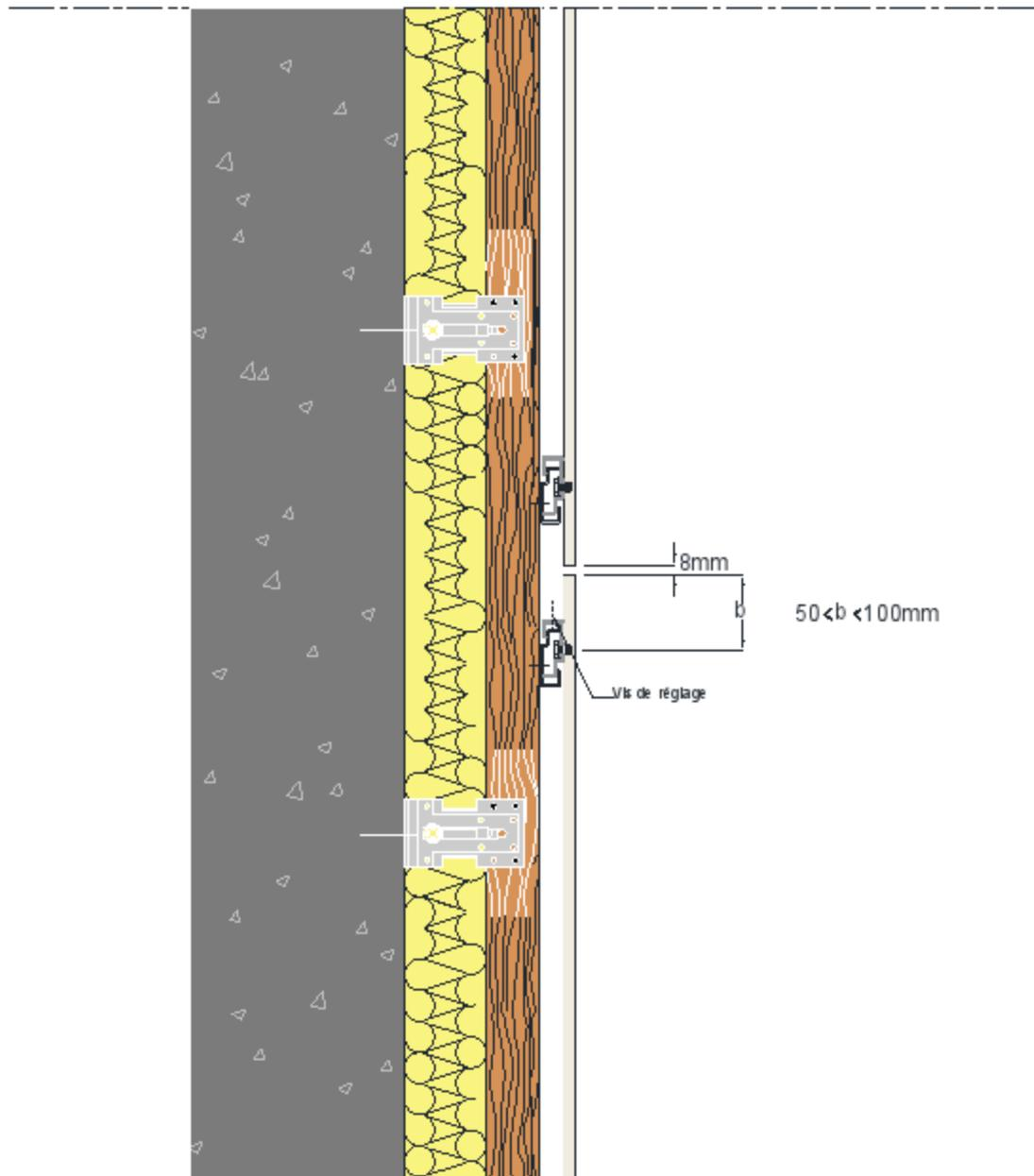
**Figure 16 – Joint Horizontal (coupe verticale)**
