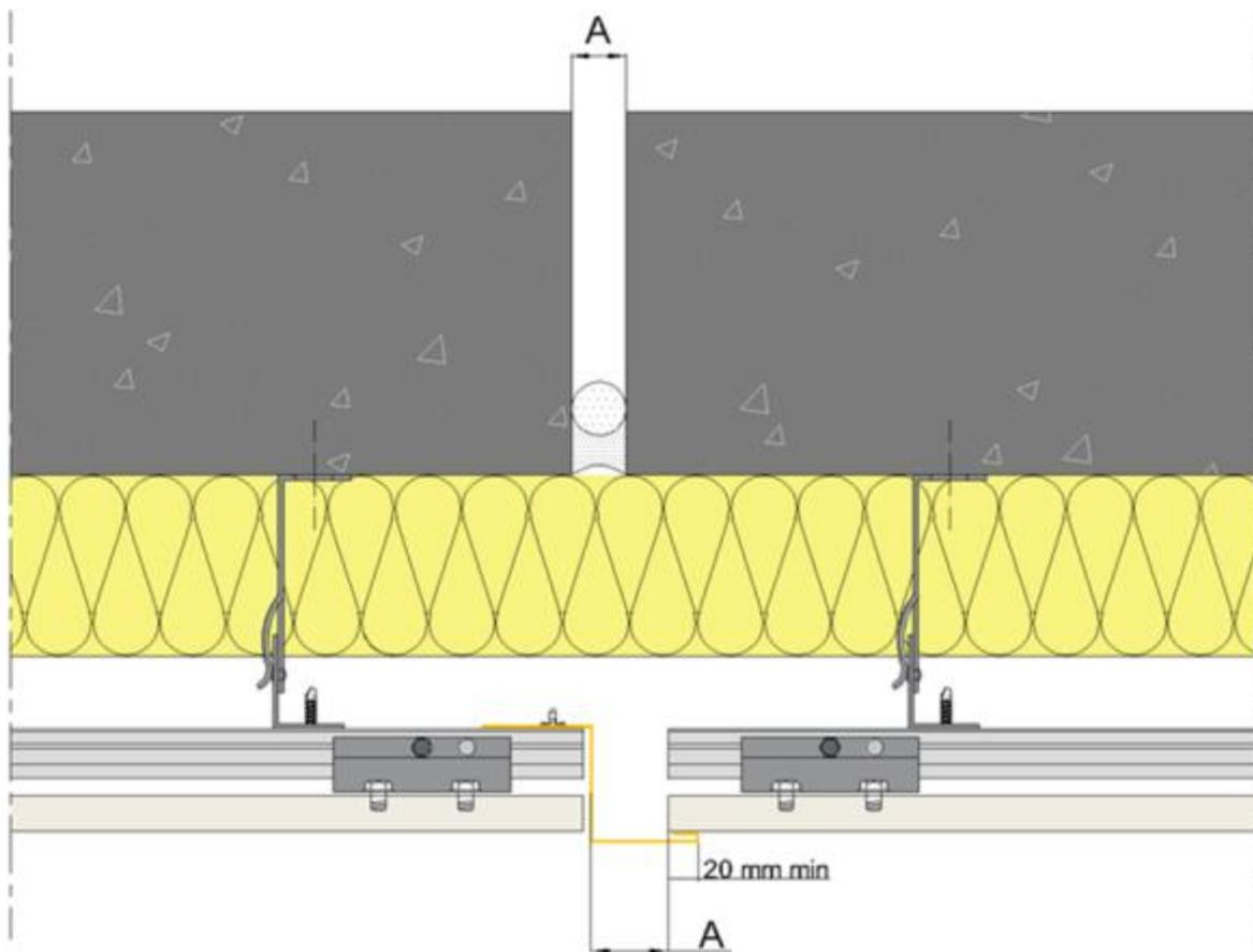
**Figure 35 - Joint de dilatation (solution 1)**
