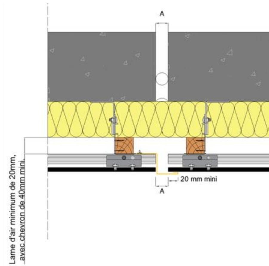
**Figure 19 - Joint de dilatation (solution 1)**
