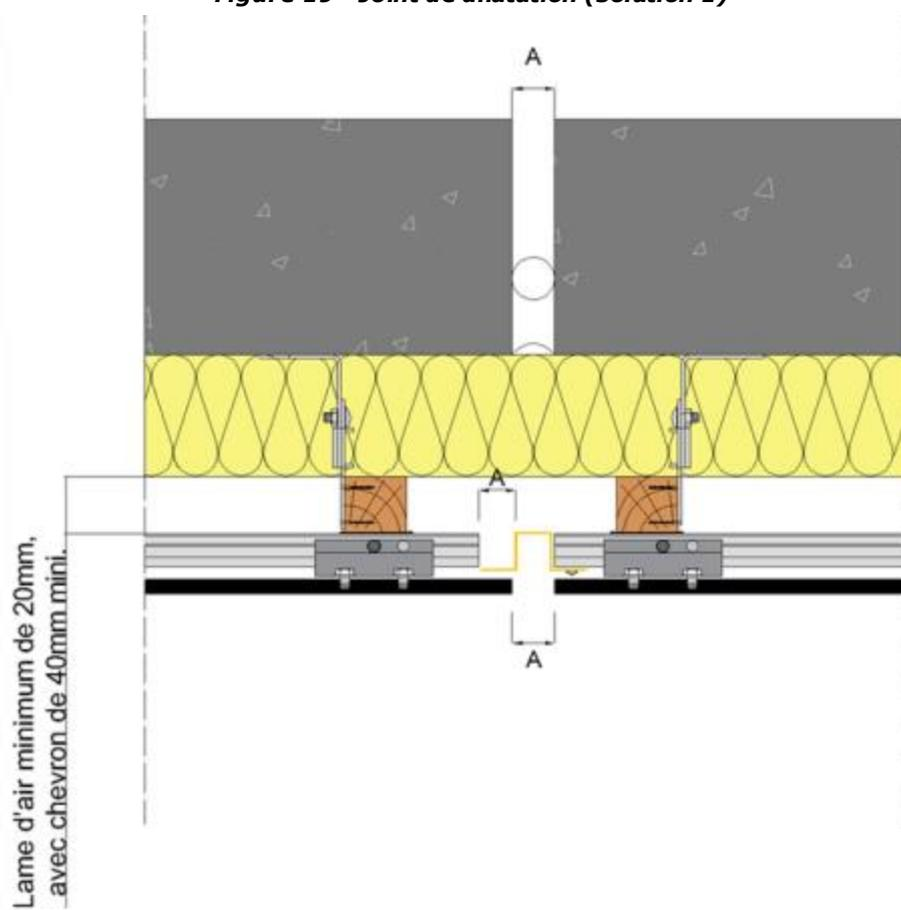
**Figure 20 - Joint de dilatation (solution 2)**
