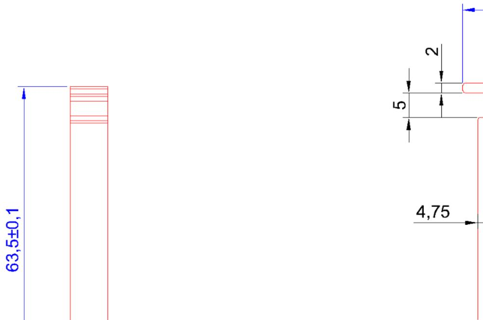
**Figure 8 - Cale de blocage KX3-Wedge**
