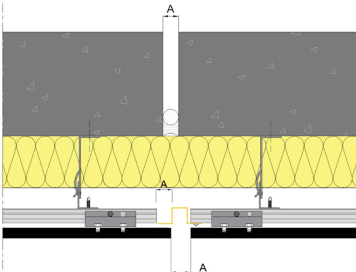
**Figure 36 - Joint de dilatation (solution 2)**
